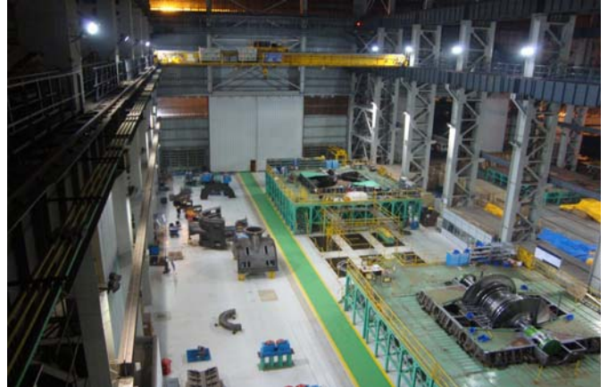
Exhibit 2: L&T – AP Genco Rotor being assembled
