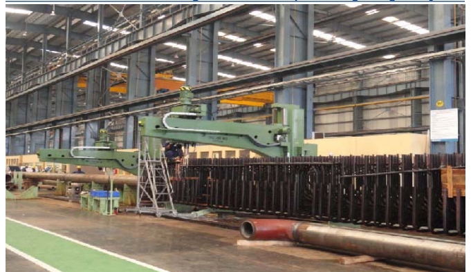
Exhibit 6: L&T - JP Power, Nigree Boiler components getting ready
