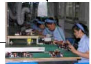
Through-hole assembly of larger odd shaped components – usually manual but can be automated
