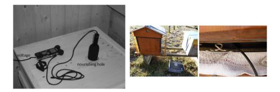
The microphone is placed either through the nourishing hole, or in the bottom part of the hive.
