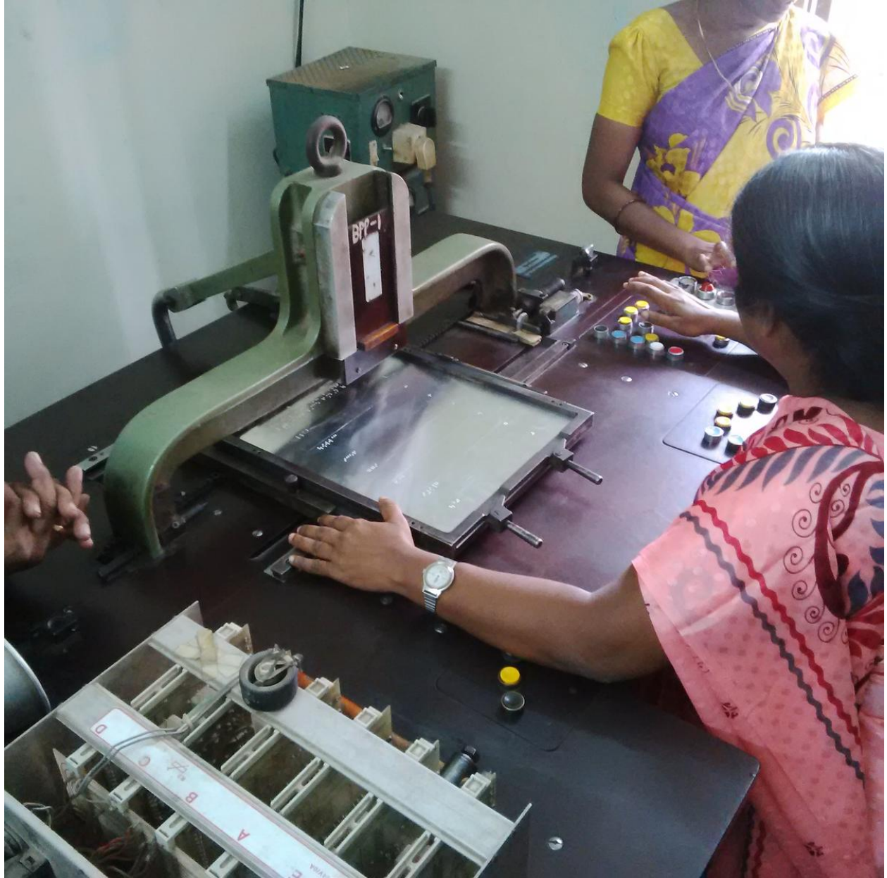
Figure 5: Stamping a page of Braille in zinc sheet
