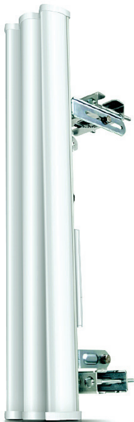
Figure 8 — Point-to-multipoint wireless link can use a Rocket M3 data radio configured as an access point, and mounted behind this Ubiquiti 3.4 GHz 120 degree sector antenna ( www.ubnt.com/airmax/airmax-sector-antenna/ ).
