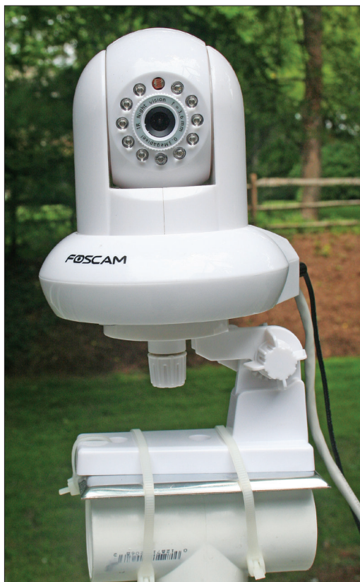
Figure 2 — A remotely controlled IP video camera can be connected to a network relay station using an Ethernet cable.
