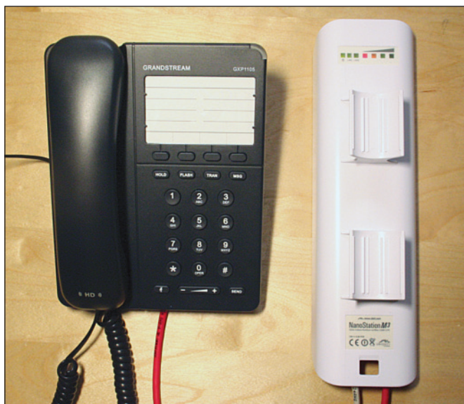
Figure 1 — This data radio station consists of a GXP1105 IP phone connected to a NanoStation M3 station by an Ethernet cable.
