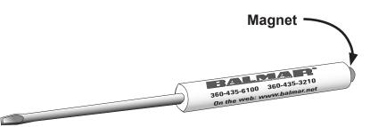
handle allows the user to activate the magnetic reed switch. By holding the magnet to the RED dot located at the end of the reed switch, the user can scroll through the regulator's various program modes and individual program selections.
