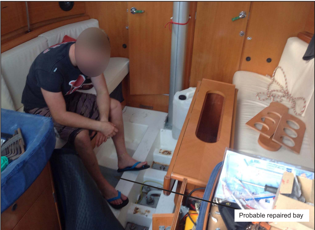
Figure 17: Cheeki Rafiki's keel bilge area prior to departure on the ARC 2013, with table temporarily removed
