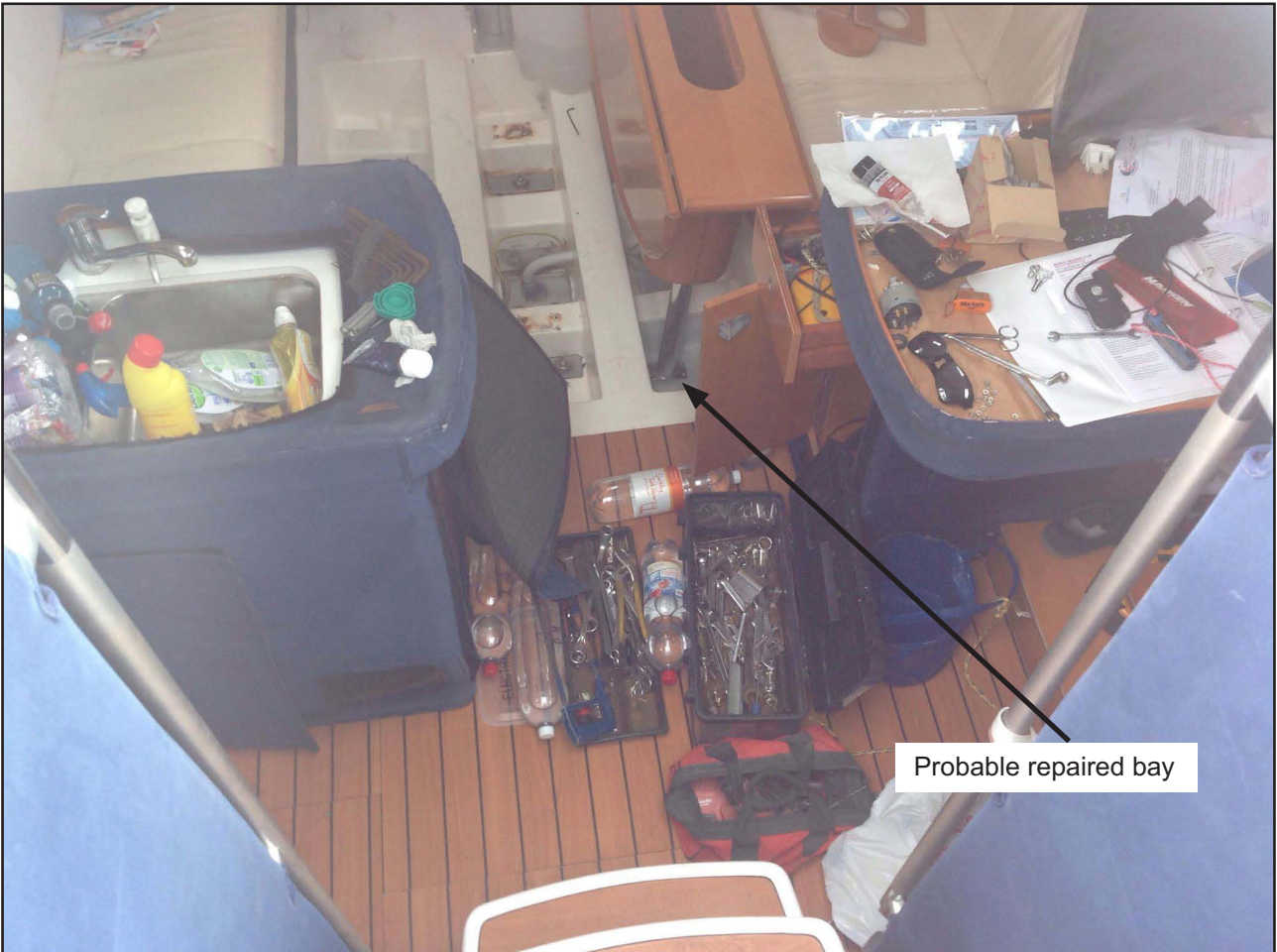
Figure 16: Cheeki Rafiki's keel bilge area prior to departure on the ARC 2013, with table temporarily removed
