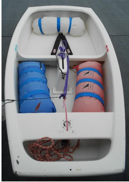
AYC #13 (MGH09312I999) 1999 McLaughlin World Champion hull in fair condition (will need fiberglass repair to port bow corner and starboard)
