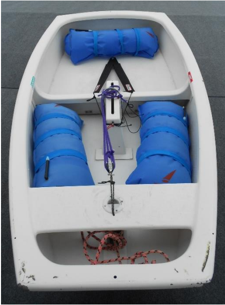
AYC #14 (MGH09381I999) 1999 McLaughlin World Champion hull in fair condition (will need fiberglass repair to mast step and bow corners)
