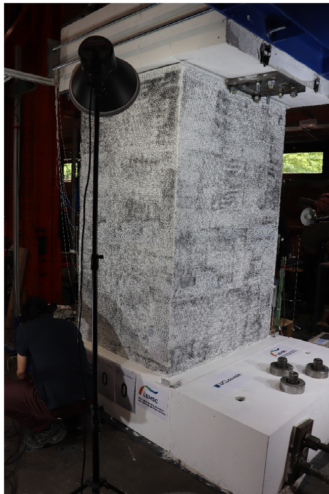
Figure 8 Speckle pattern on the East flange and Web of UW1 at LS0 (i.e., prior to loading)
