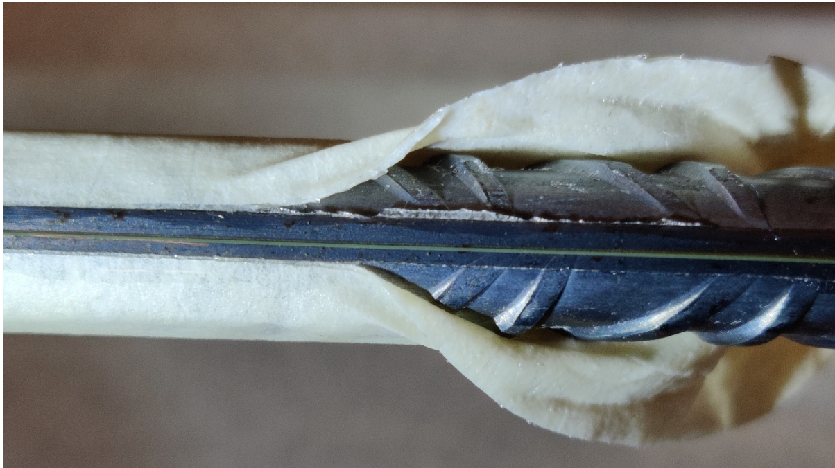
Figure 9 Close-up of the 12mm reinforcing bar with optical fiber attached
