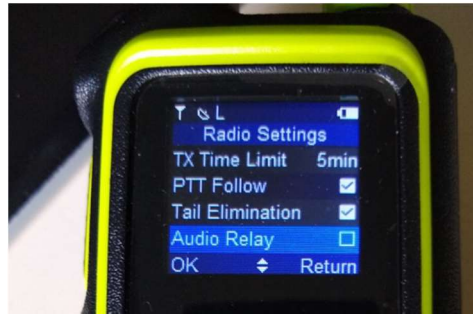
APRS & Share set to 16 Radio settings, max TX time – Audio Relay ( records signal in and plays it back )
