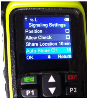
APRS & Share set to 16 Radio settings, max TX time – Audio Relay ( records signal in and plays it back )
