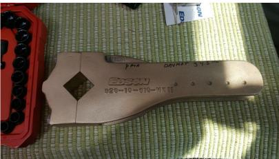
Edson 10" Bronze Tiller Arm - 34.5mm square Rudder Shaft Bore w/diagonal Fwd.
