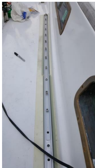
Step 4: Scribe Up-side-Down Genoa track over templates to mark out pattern on the plastic sheet!
