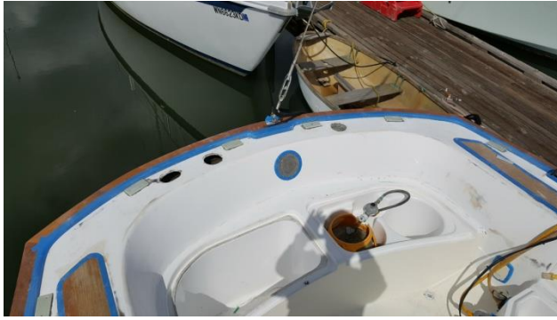
Aft rail bocks mounted.
