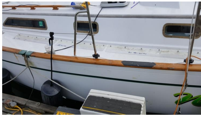
Side view of Port Templates drilled and bolted showing gate locations.
