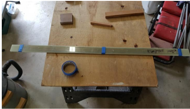
Step 7: Layout/tape template over precut 3/8" thick x 2" wide x 40" long G-10 glass
