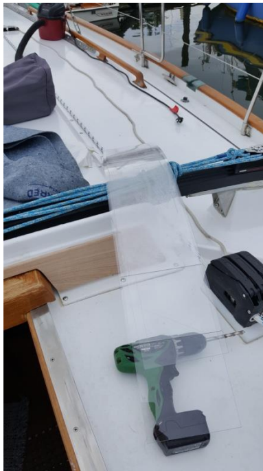
Step 1: Starts with Makrolon Plastic Template Stock
