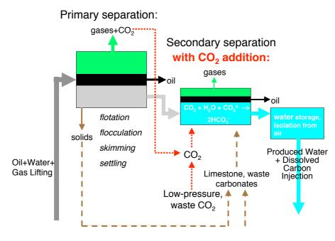
Figure 1. General scheme of water degassing, separation, and re-injection typically employed in oil production. By introducing  $CO_2$  to this water prior to re-injection, low-cost  $CO_2$  capture and sequestration can be effected. If desired,  $CO_2$  uptake can be enhanced (via reaction 1) with the addition of alkalinity, such as limestone or the carbonate solids initially precipitated from the produced water. (From Rau et al. [21]).
