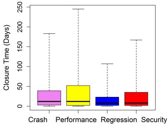
Figure 3: Boxplot for the closure time (days) for crash, performance, regression and security bugs
